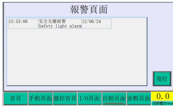
Figure 7: Safety photoelectric action screen
