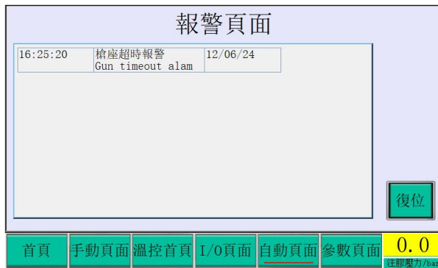
Figure 11: Cylinder Failure of Glue Gun
